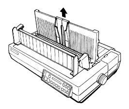
3. Tear off the sheet of labels at the perforation behind the push tractor.
